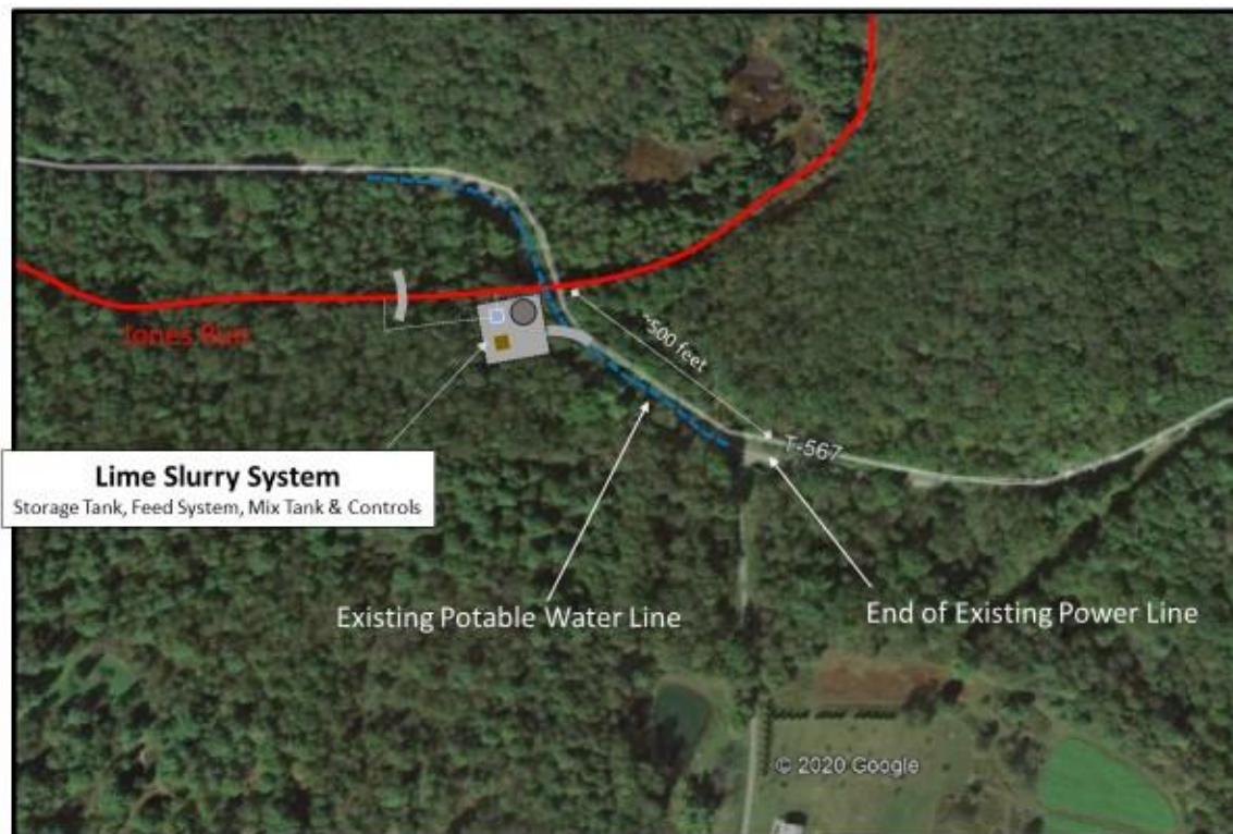
Figure 6-3. Area 1 Jones Run Conceptual Alkaline Addition Treatment System.
