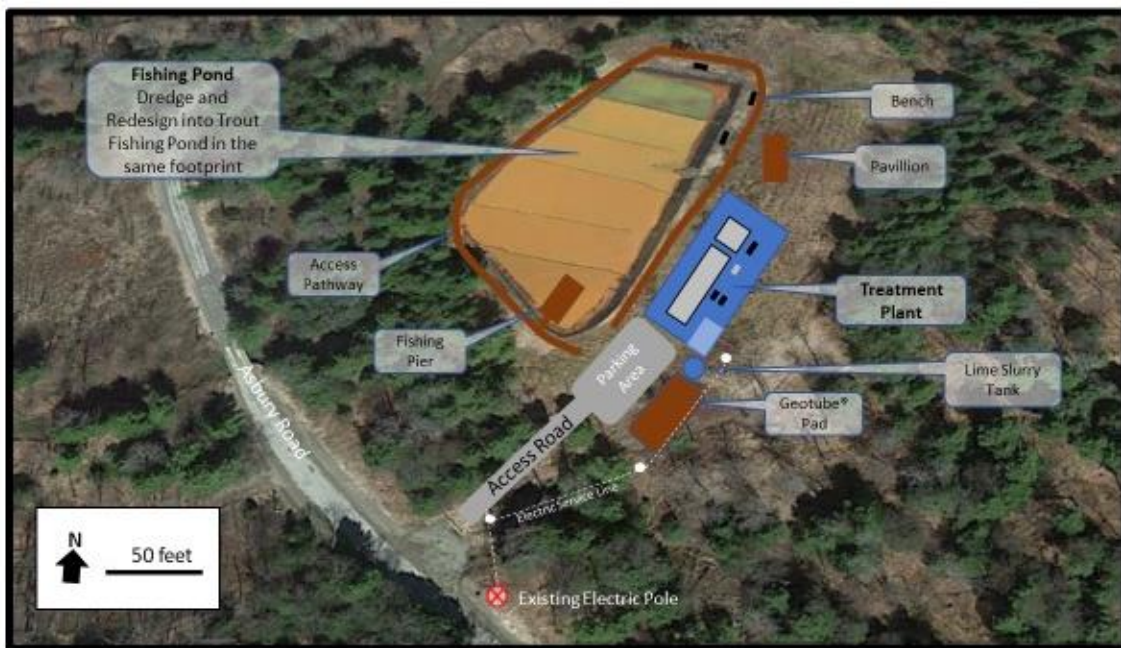
Figure 6-5. Conceptual Design of the Markel-Kotchey Active Treatment Plant & Recreational and Enhancement.
