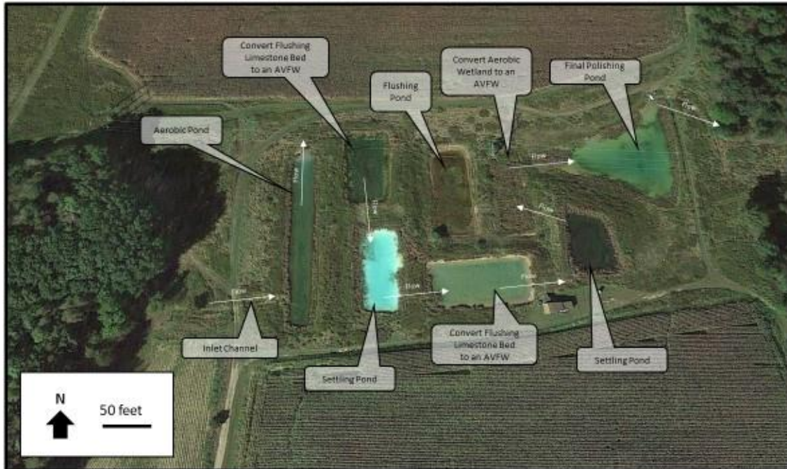
Figure 6-6. Conceptual Design for the Hanlon Passive Treatment System Rehabilitation.
