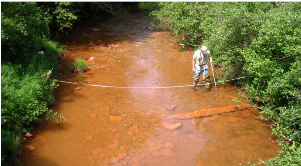
Figure 3. Little Mill below the treatment system discharge (looking downstream from the Asbury Rd. Bridge). The 60-80 mg/l of iron from the Markle/Kotchey site is diluted by Little Mill to 7-10 mg/l of iron and the pH has dropped to about 6.5.
